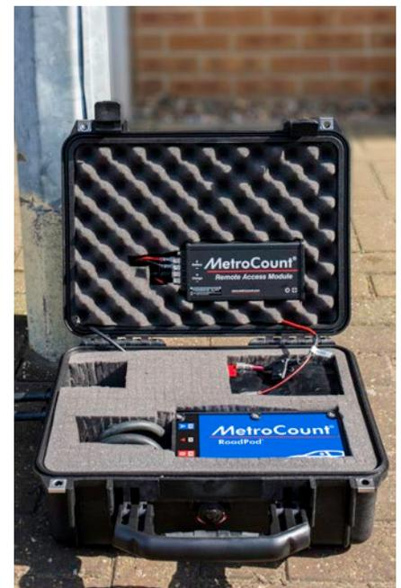
*The RidePod™ BT can be extended for FieldPod® remote access in a range of customizable enclosures like the pictured Pelican case.*
